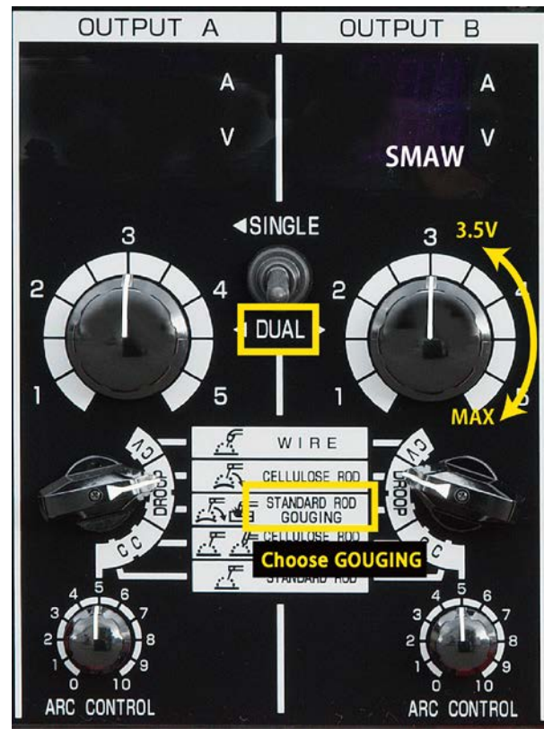
Control panel setting for SMAW
